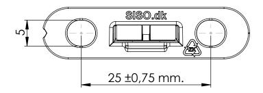
Recommended: CSK screw: head Ø8 mm. (Can be used with Euro screw)
